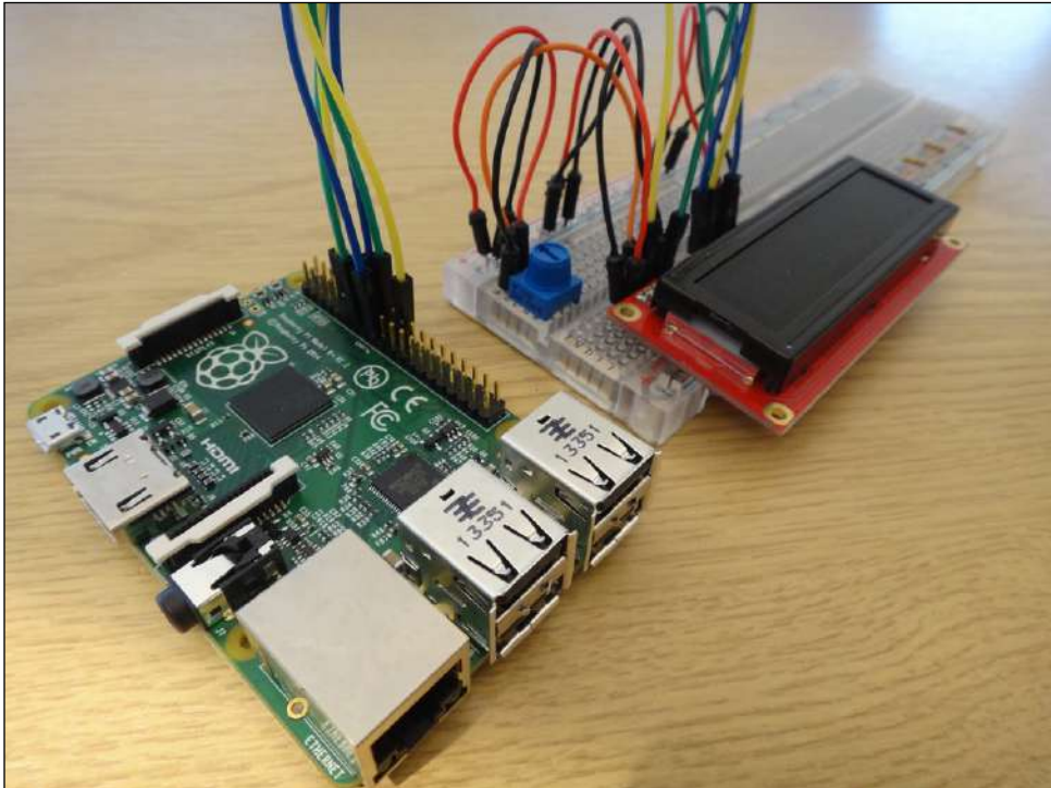
FIGURE 10-3 Mounted LCD screen and potentiometer
